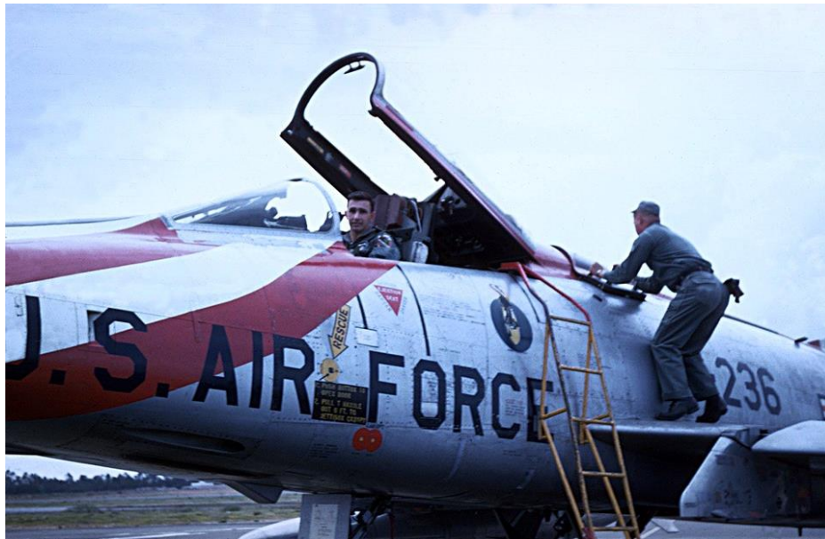
Crew Chief securing the hydraulic panel of a 494th Squadron F-100D. Chaumont, France. 1959
